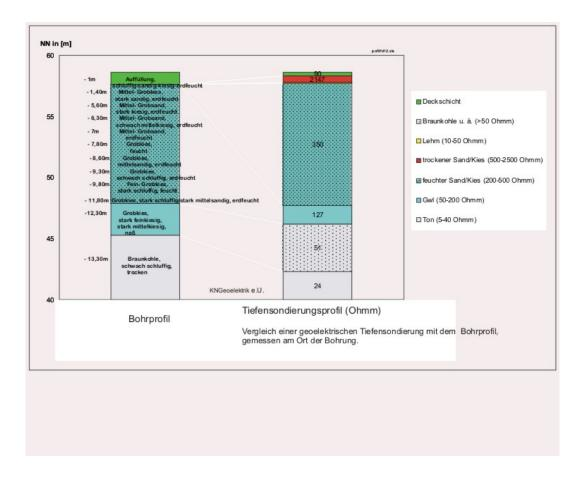
ERT: The result of the Analysis and subsequent interpretation can be adjusted by an additional well log on subtleties.
