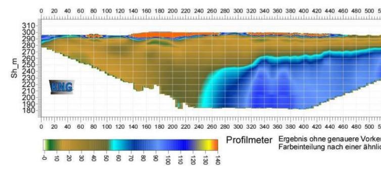
With subsequent drilling (drilling profile) resistors of aquifers and other objects can be verified.
